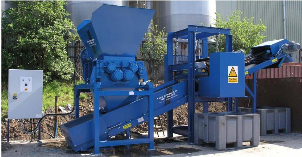
For higher throughputs and larger tyres such as truck tyres, then our TP300S/TS100 system is the system to look at. For processing of truck tyres the DB30 Tyre Debeader is required at £33,950.00. The TP300S/TS100 system includes TP300S pre-shredder with transfer conveyor to the TS100 shredder, discharge conveyor, over band magnet and rare earth drum magnet. The price for the TP300S/TS100 is £412,945.00.
